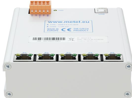
Industrial managed switches LAN-RING equipped with Ethernet ports. Event management, which is part of advanced management, makes these switches the ideal solution for applications with high demands on security and flexibility of the devices used. The switches support redundant MESH topologies with fast connection recovery. Thanks to the highly resilient hardware, the switches can be deployed in a wide operating temperature range of -40 to 70 °C.
