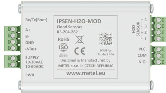
The H2O system contains components for water leak detection. The system can operate completely autonomously with an output to a local relay or it can be connected to a Modbus-RTU bus and communicate with a PLC that sends alerts, for example via SMS.
