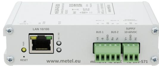
Dual channel converters 1x RS485, 1x RS232 serial port to LAN. The converters support Modbus RTU/TCP protocols (TCP-server and client). The converters are also compatible with ASSET, Galaxy Dimension alarm systems.
