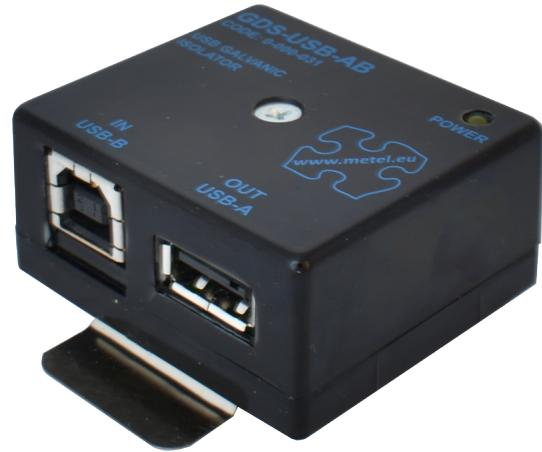
This isolator is the ideal solution for breaking ground loops and protecting USB ports from surges and voltage spikes in applications that require high-speed USB transfers. The galvanic isolation barrier can withstand potential differences of up to 2,500 V.
