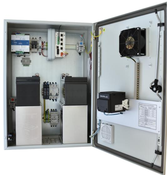
The OH7525 series outdoor steel switchboards are designed for outdoor installation of 2G and 20G series industrial switches. Models are available with a backup power supply. A Wiring Diagram and Unit Test Report are included.
