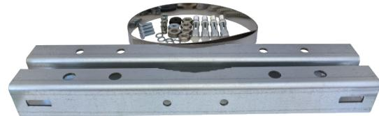
Brackets for pole mounting of OH series switchgear are made of coated steel profiles. The package also includes stainless steel bands and clips of the Bandimex system, which guarantee a safe attachment of the switchboards to the poles.
